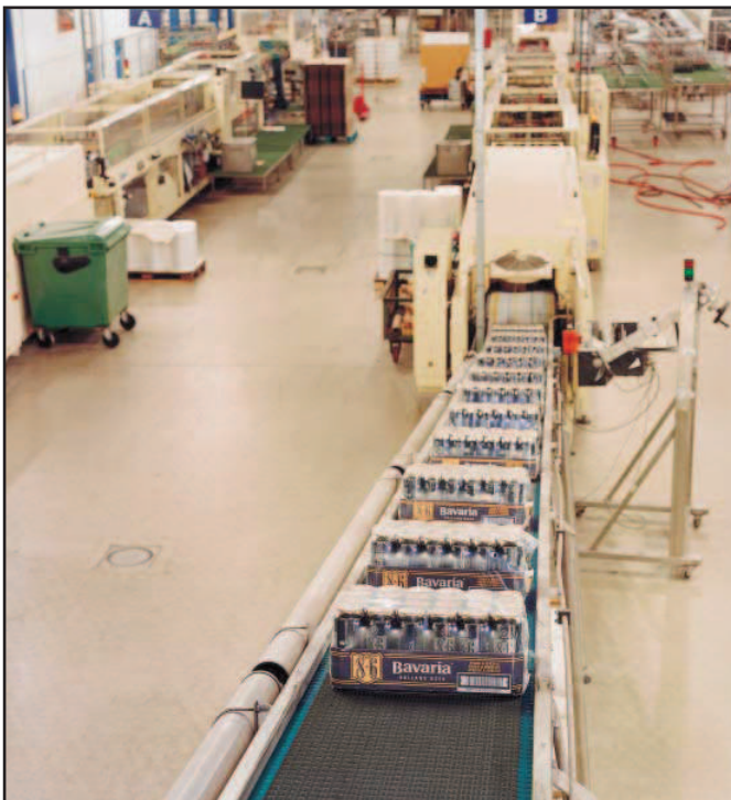
TRAY CONVEYOR WITH 1005 SUPERGRIP BELT
