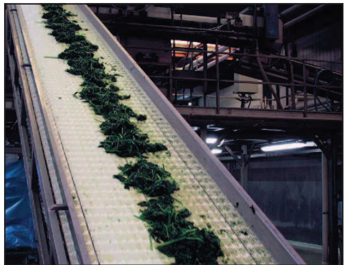
SPINACH ELEVATED ON 6391 MATTOP CHAIN
