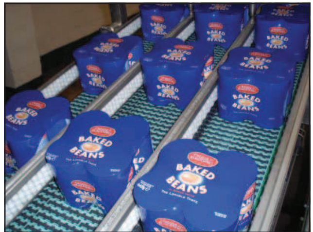
CONVEYOR WITH SGDP1505 XP BELT
