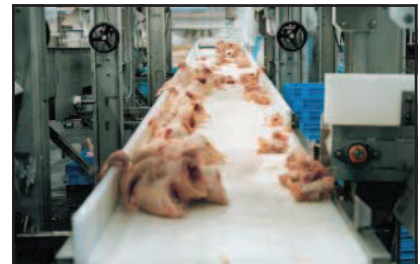
CHICKEN DEBONING LINE WITH 2015 MATTOP CHAIN
