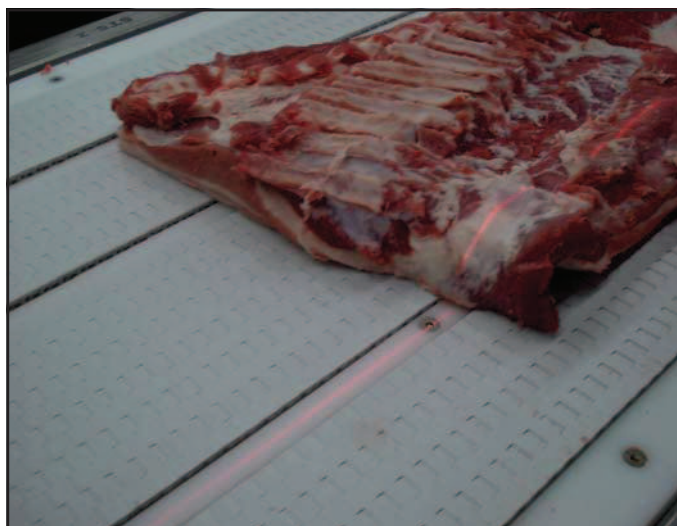
CONVEYOR WITH 515 BELT
