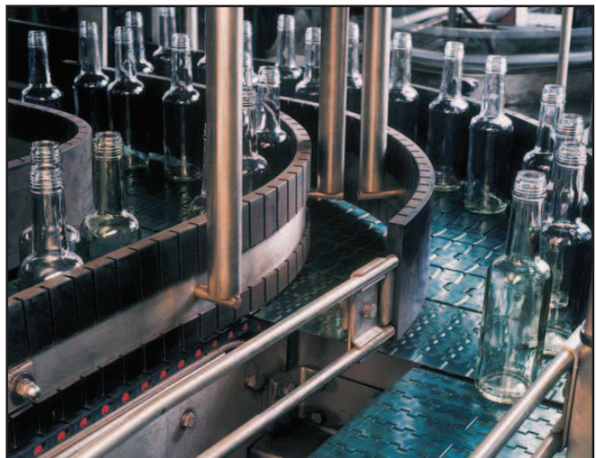
GLASS BOTTLE MANUFACTURING ON 1005 FLAT TOP BELT
