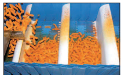
INFEEED OF INCLINED CONVEYOR WITH 2010 ISR6
