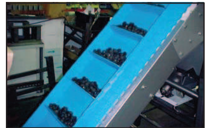
CONFECTIONARY ELEVATING ON 2015 MATTOP CHAIN
