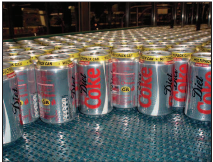
CONVEYOR WITH 500 BELT
