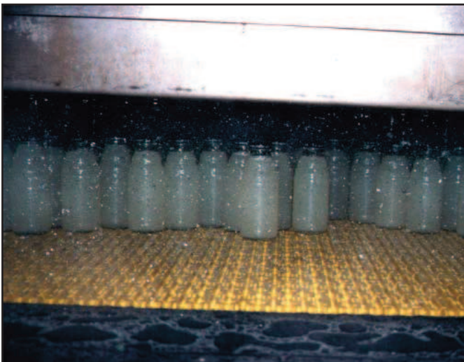
BOTTLE PASTEURIZER INFED WITH 2500 BELT
