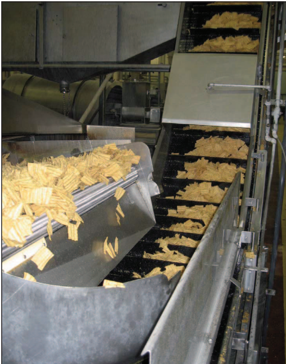
INCLINED CONVEYOR FOR CHIPS FTR2015 MATTOP CHAIN
