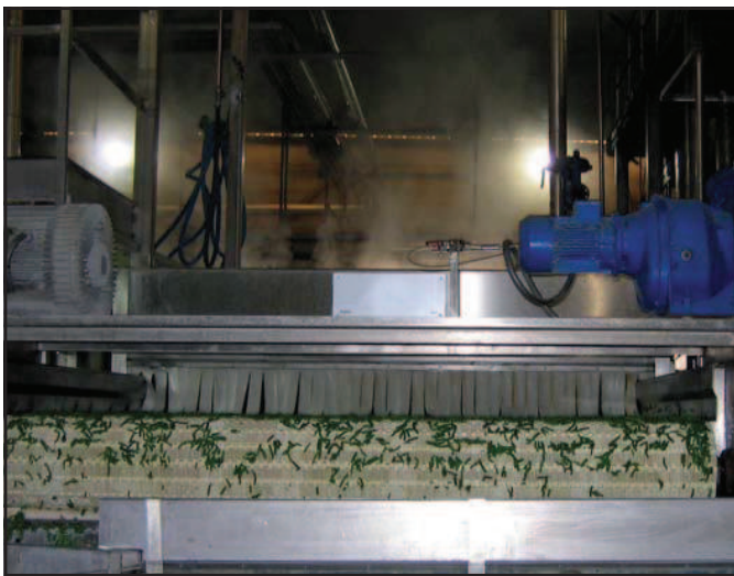
BEANS BLANCHER WITH 6391 MATTOP CHAIN
