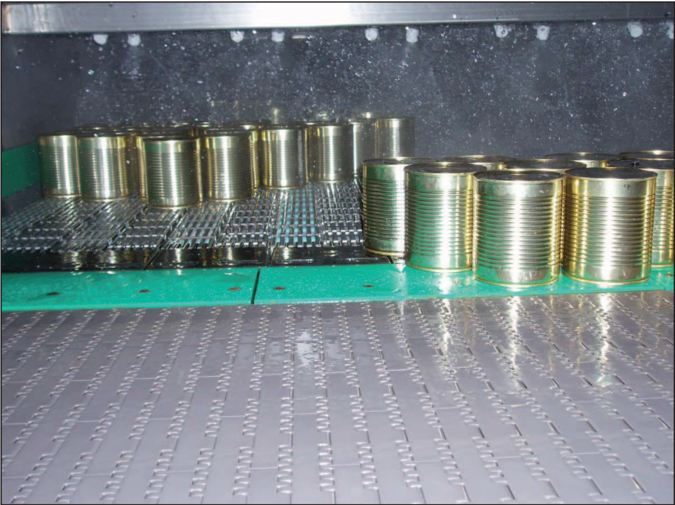
FORTREX 9227 BELT IN A FOOD TUNNEL PASTEURIZER
