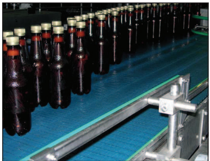
BOTTLES CONVEYOR WITH FTDP1000 XLG MATTOP CHAIN
