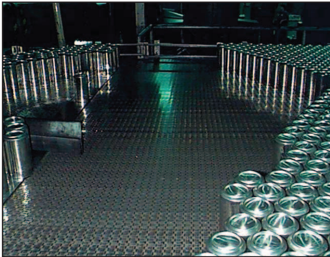
CAN WASHER DISCHARGE WITH 5936 BELT
