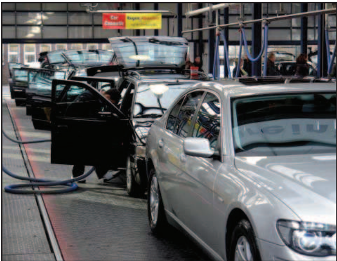
CAR INTERIOR CLEANING (DETAILING) INSTALLATION WITH 6995 BELT
