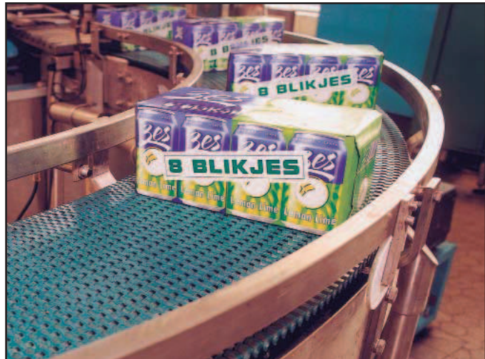
PACK CONVEYOR WITH 505 BELT
