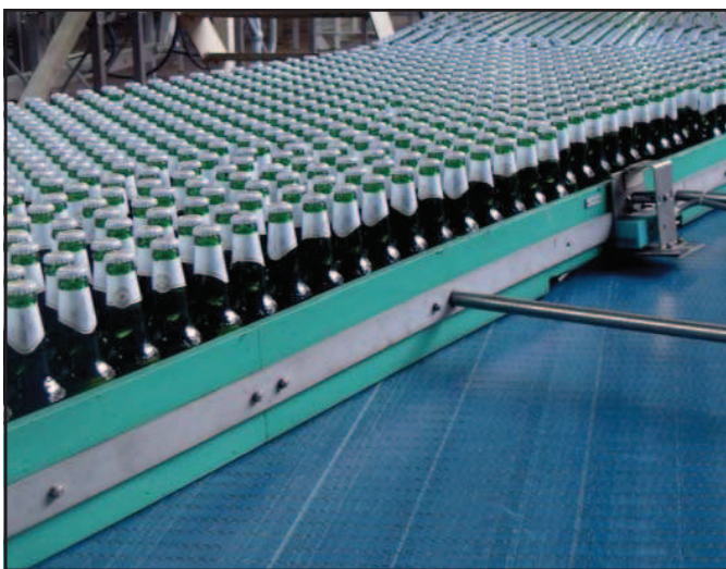
BOTTLES CONVEYOR WITH FT1000 XLG MATTOP CHAIN
