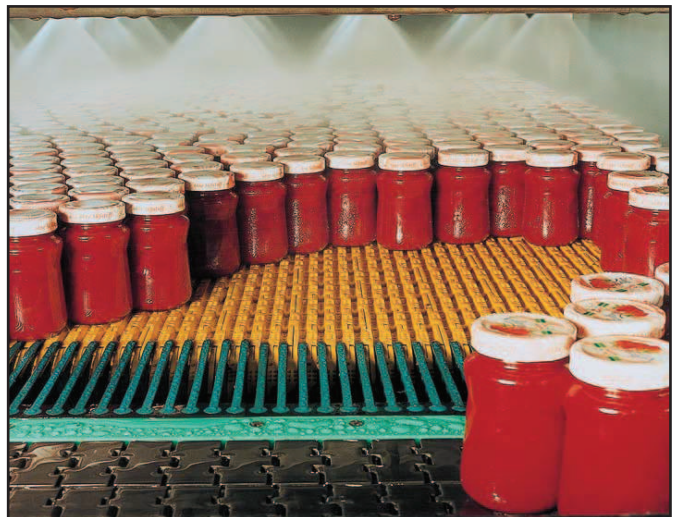
GLASS JARS PASTEURIZING ON 2500 BELT
